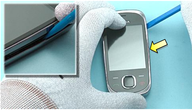
7) Use the SS-93 to release the clip holding the slider module.
