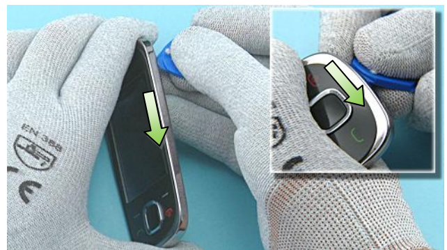
22) Slide the SRT-6 between the A-COVER and the slider module to release the side and the bottom end of the A-COVER.
