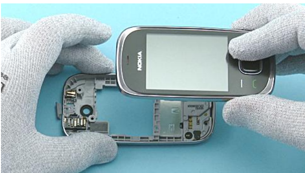
9) The D-COVER can now be separated from the rest of the device.
