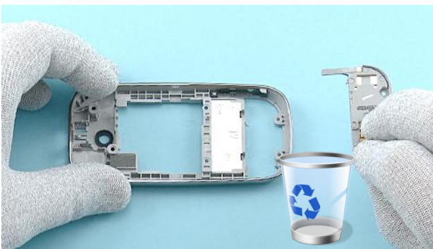
21) Remove the ANTENNA MODULE. Do not use it again. Discard it.
