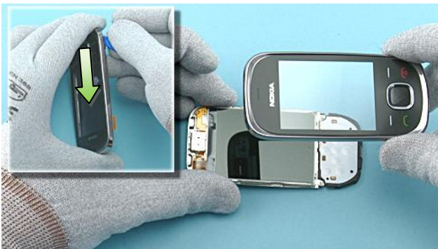
23) Release also the other side of the A-COVER with SRT-6. Lift up and remove the A-COVER.
